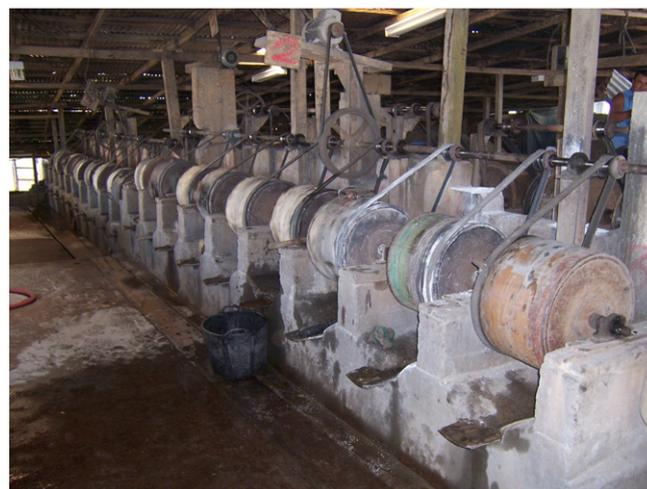
Fig. 2. Cocos are small ball mills to grind and amalgamate the whole ore.
