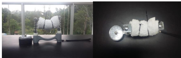
Figura 3. Dinamómetro manual Jamar Hydraulic Hand Dinamometer (JHHD)
