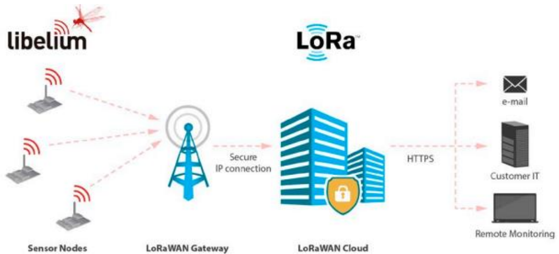
Figura 5. Red LoRaWAN. Fuente: Waspote LoRaWAN, http://www.libelium.com/downloads/documentation/waspote-lorawan-networking-guide.pdf
