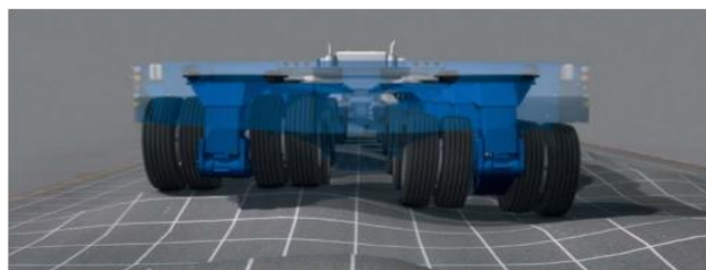
Hydraulic axle suspension – lateral + lateral swing movement
