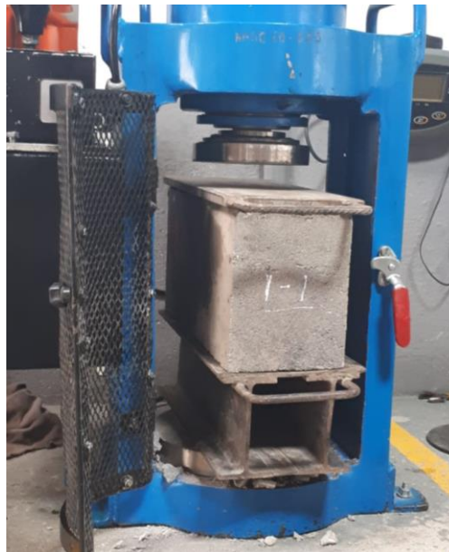
FIGURE 3. COMPRESSION STRENGTH TEST SCHEME FOR CONCRETE BLOCKS.
