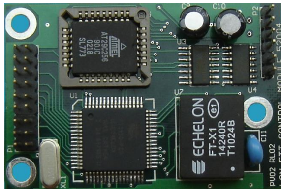
Figura 86. Módulo de control de LonPoint. ( http://www.lonworks.org.cn/en/index.html )
