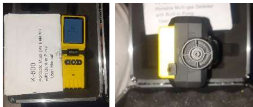
Medidor, detector portátil de gas H 2 S y CH 4 (Portable Multi-gas Detector with Built-in Pump).
