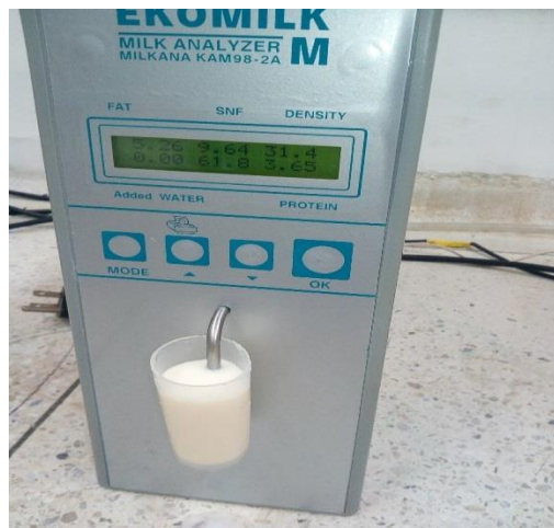
Figura 3. EKOMILK M Milk Analyzer Milkana KAM 98-2A . Foto del autor.
