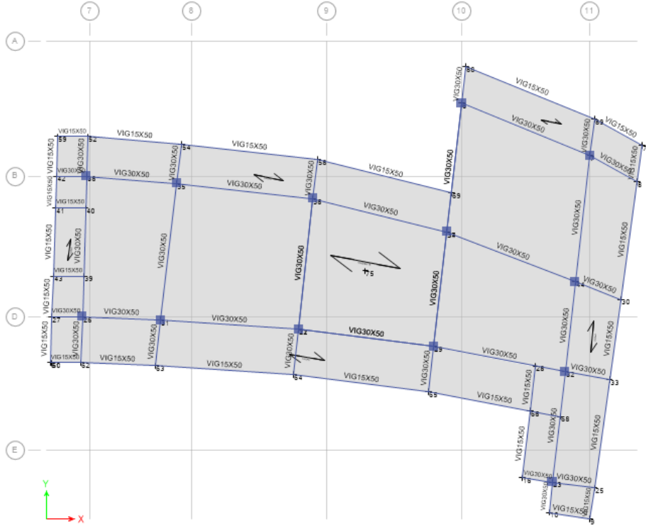
Plan View - Story5 - Z = 17.1 (m) Joint Restraints
