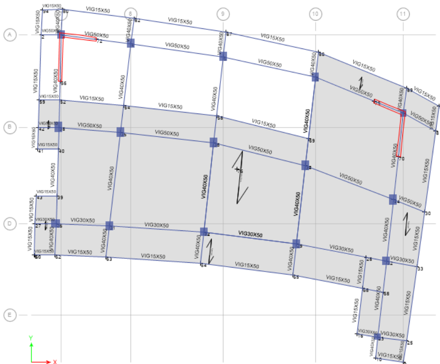
Plan View - Story4 - Z = 13.8 (m) Joint Restraints
