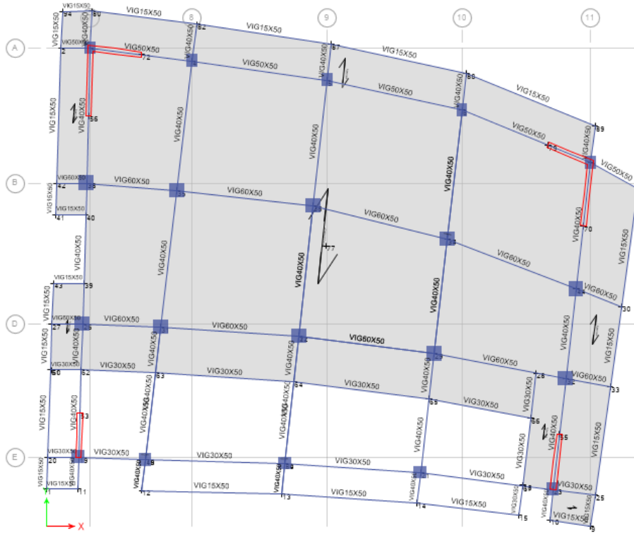
Plan View - Story3 - Z = 10.5 (m) Joint Restraints
