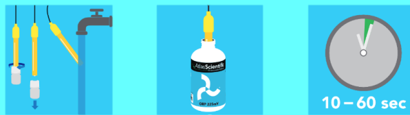
Figure 26. ORP probe calibration process [5].
