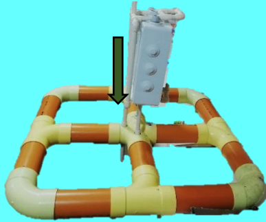
Figure 12. Anchoring support structure to floater.
