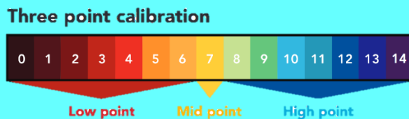
Figure 25. pH range with three point calibration [4].
