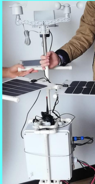
Figure 5. Weather station above support structure.
