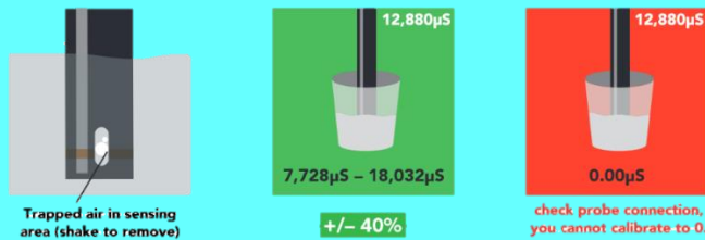
Figure 27. EC probe calibration process [6].
