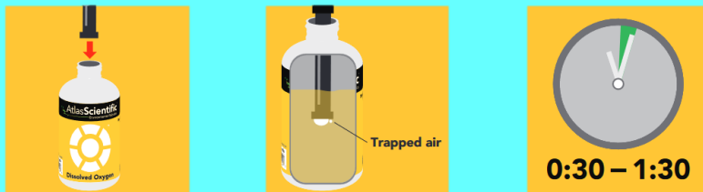
Figure 28. DO probe calibration process [7].
