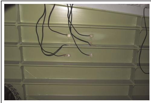
Figure 7. Sections tested with the PZT location.
