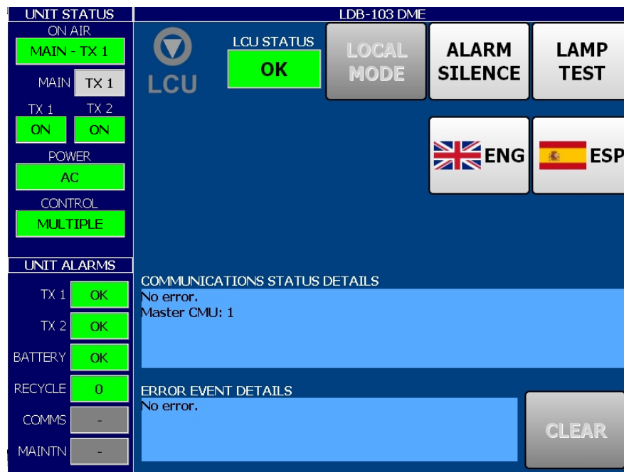
Figure 7.3.2.4-2. LCU SCREEN - LCU STATUS SLIDING PANEL INFORMATION
