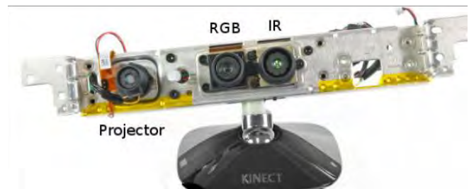
Fig. 1. Partes del Sensor Kinect. Autor: J. Smisek, M. Jancosek, and T. Pajdla, "3D with Kinect.
