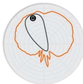
Figure 4. R510 2.4GHz Elevation Antenna Patterns
