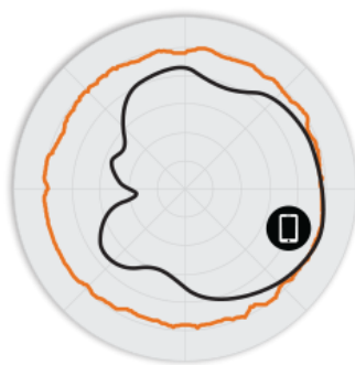
Figure 3. R510 5GHz Azimuth Antenna Patterns
