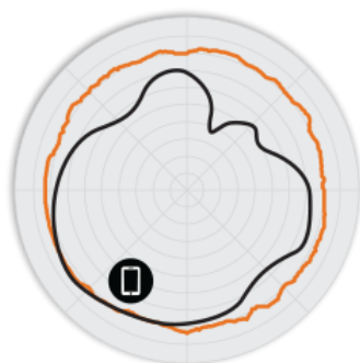
Figure 2. R510 2.4GHz Azimuth Antenna Patterns
