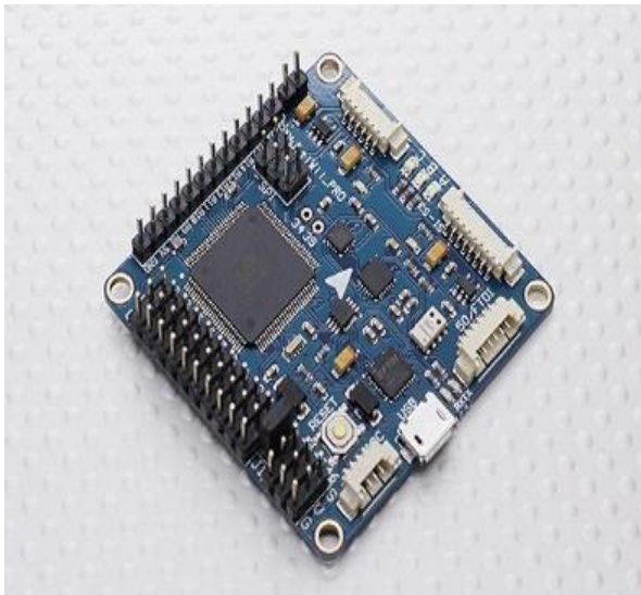
Figura 5. Tarjeta de Control de Vuelo Multiwii All in One PRO 2.0v. Recuperado de (“Multiwii and Megapirate AIO Flight Controller w/FTDI (ATmega 2560) V2.0 (US Warehouse)”, 2016)
