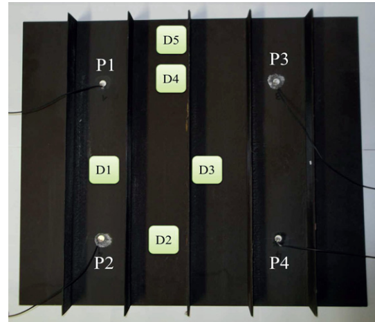
Figure 2. Simplified aircraft composite skin panel: setup and damage positions.
