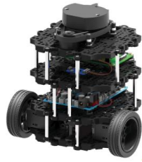
Figura 21. Robot turtlebot3 burger. Tomado de manual robotics. Fuente. TurtleBot 3 Burger. (Robots Components, 2016)
