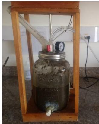
Figura 8. Reactor semicontinuo tipo fed-batch. Por: Quijano & Ramirez 2020.
