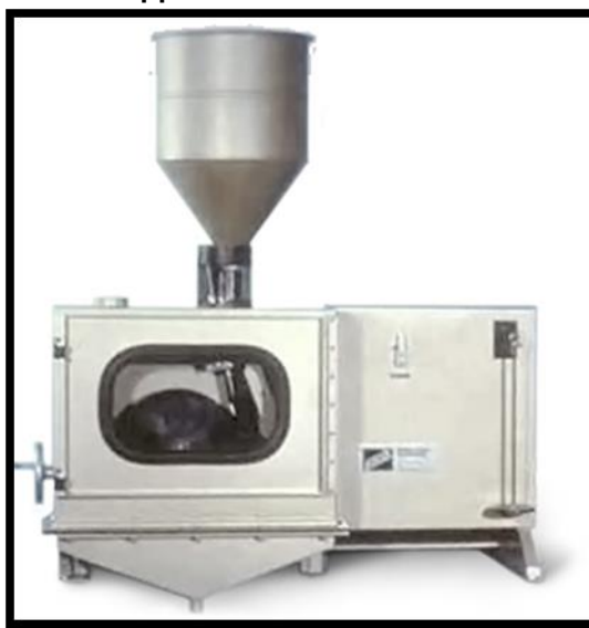
Figura 21 FALDEX - Dry rubber/sand wheel apparatus
