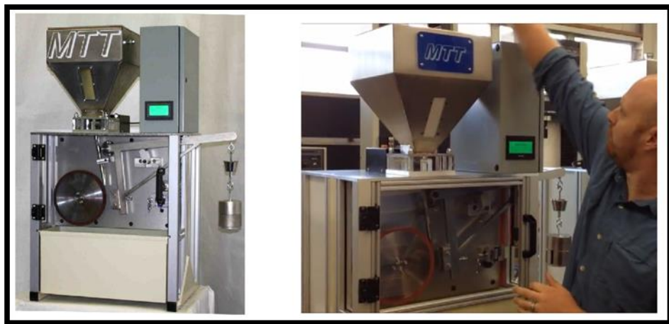
Figura 19 MTT ASTM G0065.10/ Sand Wheel Abrasion Tester
