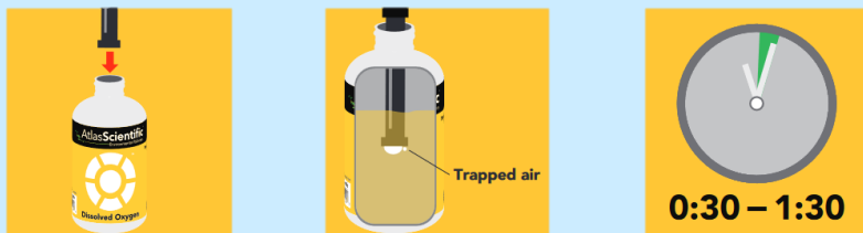
Figure 23. DO probe calibration process [8].
