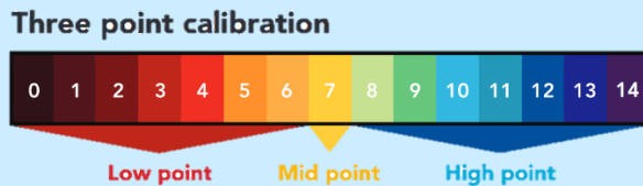
Figure 20. pH range with three point calibration [5].
