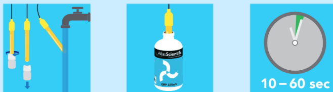
Figure 21. ORP probe calibration process [6].
