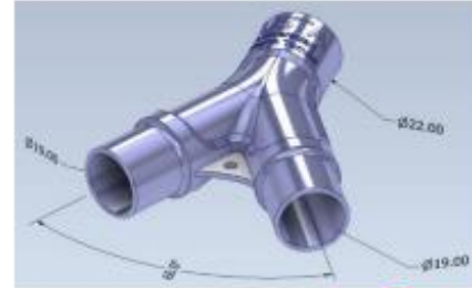
Fig. 7. Detail of the internal inlet and outlet diameters in the duplicator. Source: Authors
