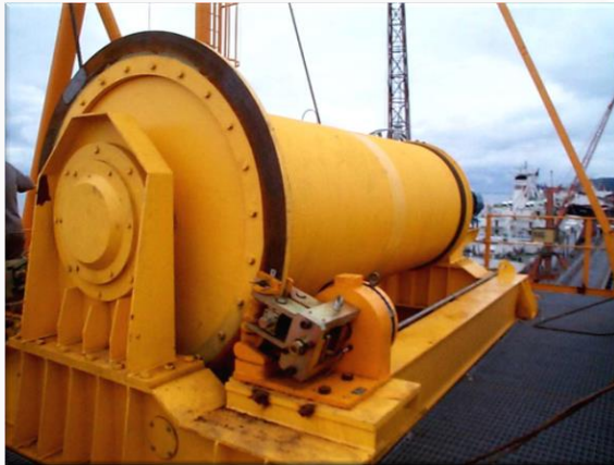
Electromagnetic Disc Brake (emergency brake) , model 10C and power supply. Braking Torque: 220.000 Nm
