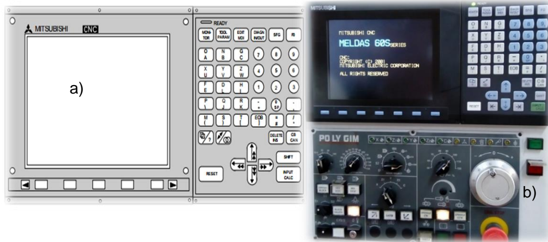
Figura 2. (a) Esquema del control Mitsubishi Meldas 60S. (b) Tablero del control Meldas 60S.
