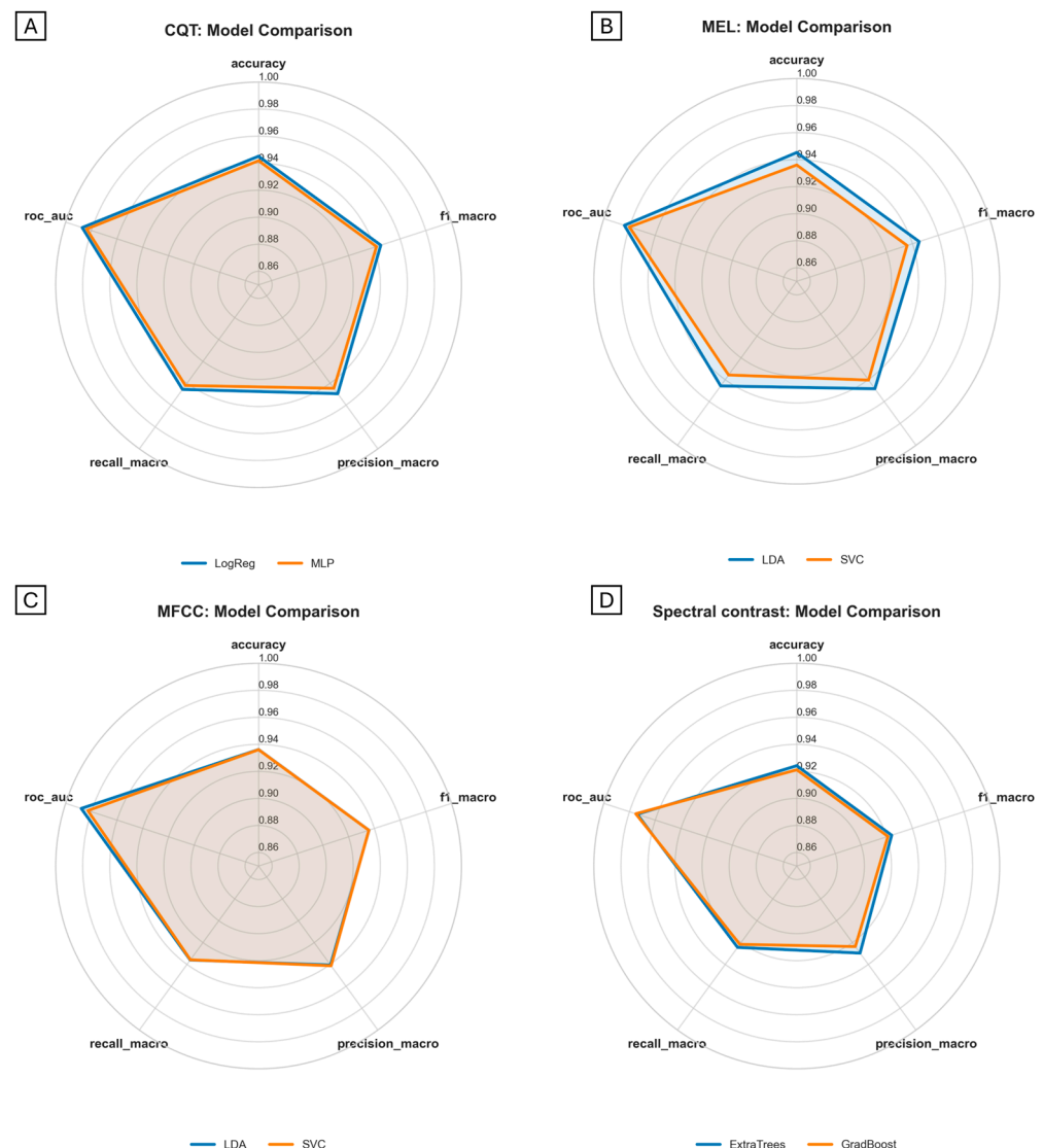
Figure 8. Performance of the top-performing models by spectral transformation. (A) CQT transformation; (B) MEL transformation; (C) MFCC transformation; (D) Spectral Contrast transformation.
