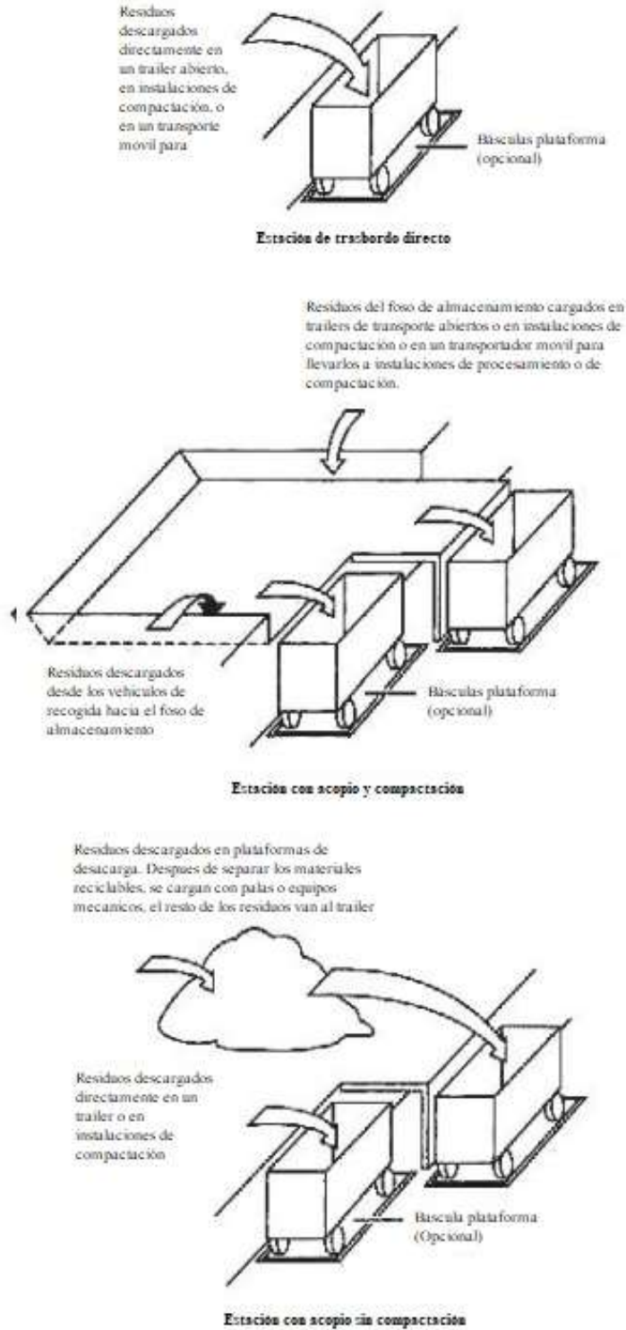
Figura 10. Esquemas de estaciones de transferencia Elaboración a partir de: (Tchobanoglous, Theisen, & Virgil, Integrated solid waste management: Engineering principles and management Issues, 1993)
