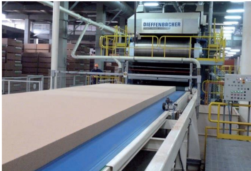
Figura 34. Prensa de rodillos para tableros aglomerados, foto: Wood Based Panels, (United States Environmental Protection Agency, 2002).
