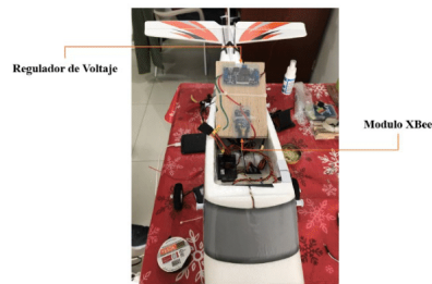
Figure 13. System fitted inside the Model Aircraft Part Below. Source : Author
